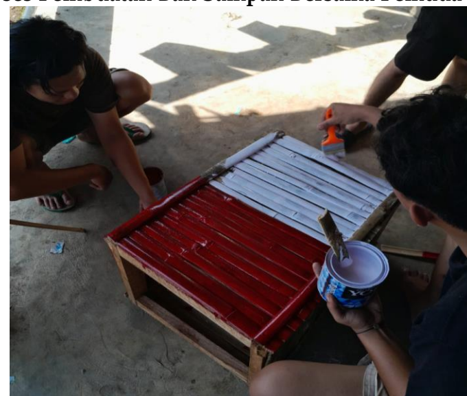
Gambar 5. Proses pengecatan Bak Sampah
